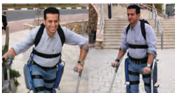
Israeli company ReWalk developed an exoskeleton to allow paraplegics to stand, walk, and climb stairs.
